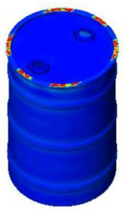
stresses in a plastic product were located at this zone because of deformations are recoverable when load ceases. However, sometimes it is necessary to perform an analysis loads where or deformations exceed such status. A simple elastic-linear analysis can be used in order to calculate stress or deformation of any part that shows a non-linear elastic behavior. It is only
