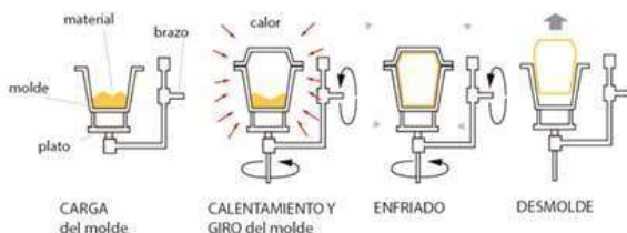
Figure 4. Rotational molding process.
