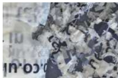
Figure 11. Effect of oxodegradable additive in the appearance of plastic bags.
