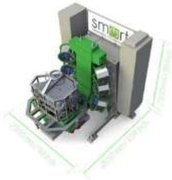
Figure 12. Persico rotational molding machine.
