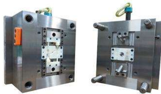
Figure 9: Molds from Hasco with 3D printed plastic inserts [taken from web page blog.stratasys.com ].
