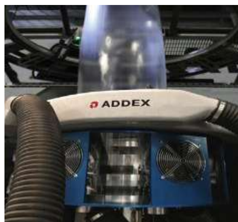
Figure 6: Cooling ring system ICE of Addex [taken from "Film, Sheet and Extrusion" magazine, November 2016].
