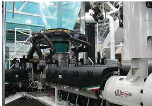
Figure 8: POD extrusion line of Macchi for stand-up pouches manufacturing [taken from "Film & Sheet Extrusion" magazine, October 2016].
