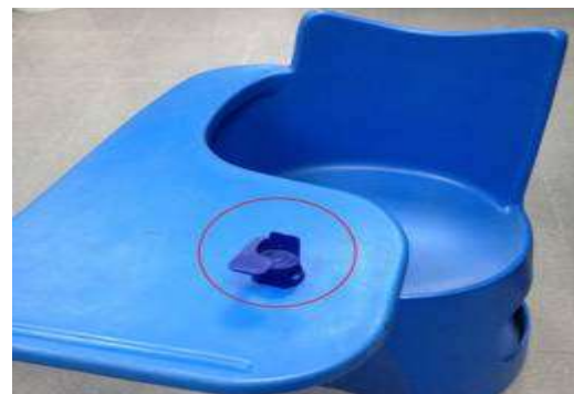
Fig. 13 Desk prototype created by 3D Printing at Indesca
