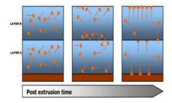
Based on this mechanism it can also be anticipate that those extrusion lines, coextrusion, lamination, cutting, among others, which have central tension winders, will have a heterogeneous distribution of slip agent with higher COF in the center of the roll.
