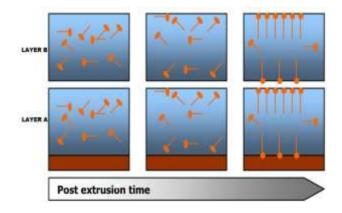
In the precedent representation, the slip-agent molecules move towards the free surfaces of the film, allowing the polar group of amide molecule, incompatible with PE, to forms the slippery film. As there is no excessive pressure on the winding, the amide remains on the surface and does not migrate.
