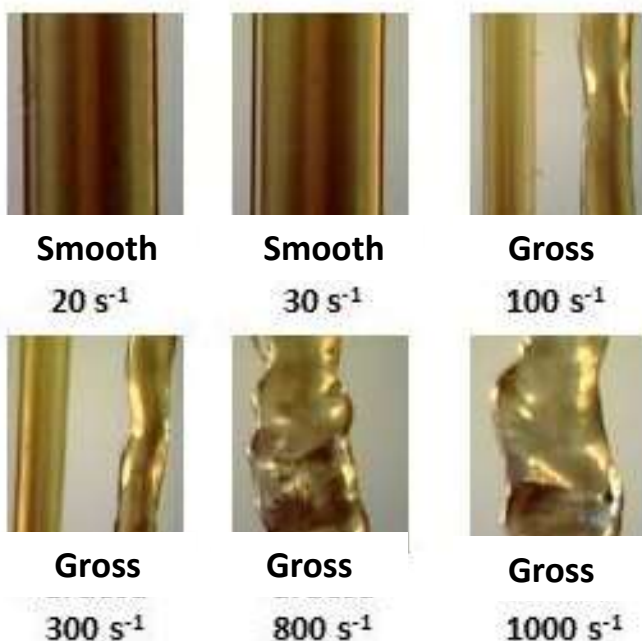
Figure 6 LDPE melt fracture at different shear speeds in a capillary rheometer (11).
