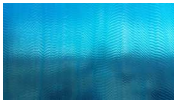
Figure 5 Photograph of melt fracture of a LLDPE extruded film.
