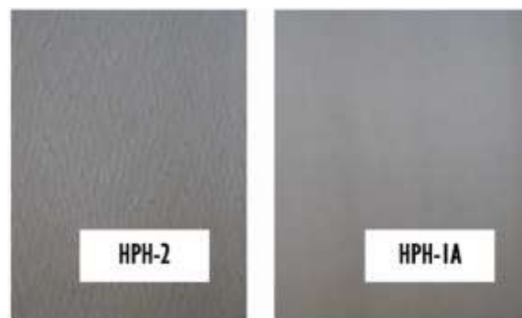
Figure 4 Examples of films with extreme melt fracture (HPH-2) and no melt fracture (HPH-1A)
